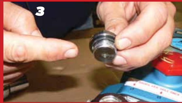
3 Examine the O-Ring under the Valve Plug for cuts or distortion and replace if worn. Lubricate the new O-Rings before installing on the manifold.
