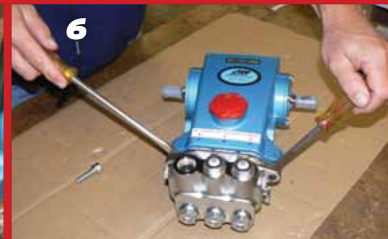
6 Separate Manifold Head from crankcase by turning the shaft, insert 2 screwdrivers in gap and pry Manifold Head forward until it comes off.
