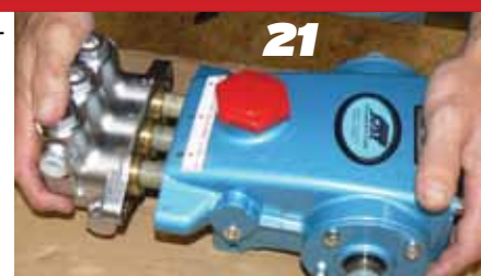
Install the Seal Retainer with new Wick onto each plunger rod with tab down and wick out . Replace two Lockwashers, two Socket Head Screws for four Flange Nuts and torque.
