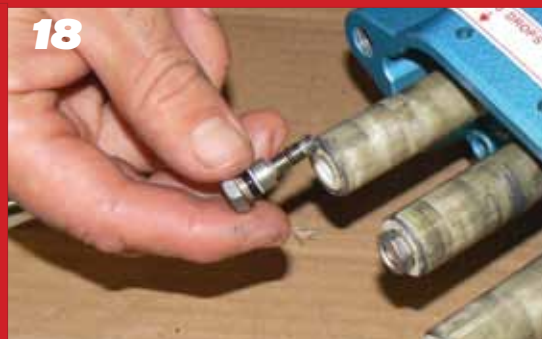
Install new Gasket, then O-Ring, then Back-Up onto each Plunger Retainer.
