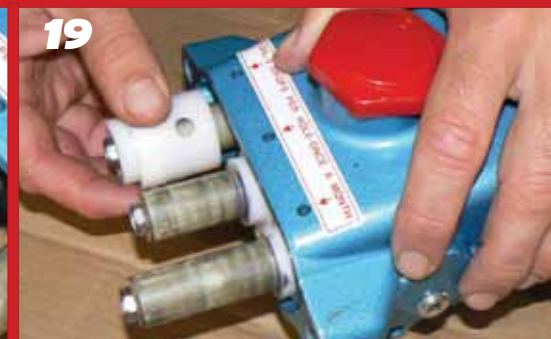
Install the Seal Retainer with new Wick onto each plunger rod with tab down and wick out . Replace two Lockwashers, two Socket Head Screws for four Flange Nuts and torque.
