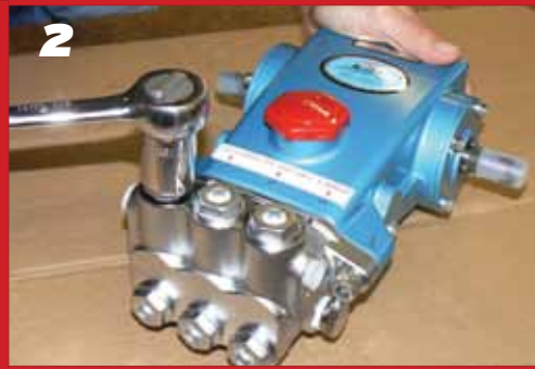
2 Remove the hex Valve Plugs (top discharge, bottom inlet)
