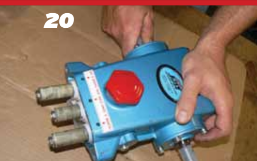
Rotate Crankshaft by hand so the two outside plungers are extended equally.
