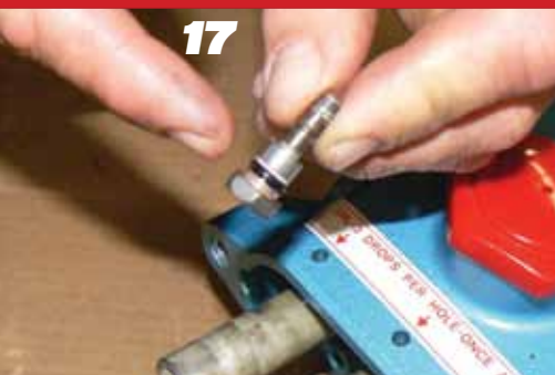
Inspect O-Ring and Back-Up Ring for wear & replace if needed. Examine Ceramic Plunger for scoring, scale build-up, chips or cracks and replace if needed.
