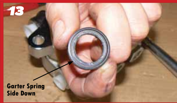
Lo-Pressure Seal must be installed with Garter Spring side down . The down direction is facing the front of the manifold.
