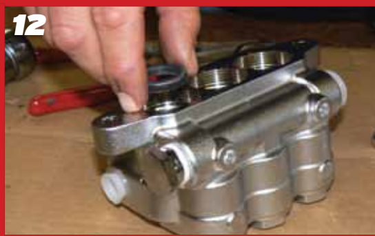
Examine Seal Case O-Ring and replace if worn. Lubricate new O-Ring before installing.
