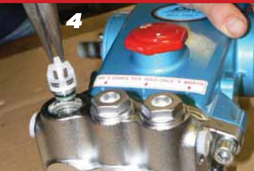
4 Grasp Spring Retainer by tab at the top with pliers and remove from valve chamber.
